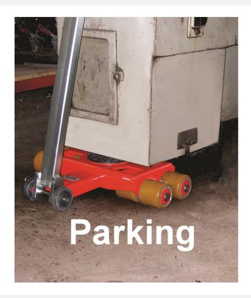
You can leave your load sitting on top of the dollies for extended periods of time. This will not damage the dollies or rollers. The rollers will begin to sag until the load starts moving, and then the roller material will return to its original shape.
