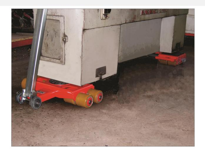
**Step 5:** Now push the load. The pulling handle can also be hooked to a forklift for towing.
