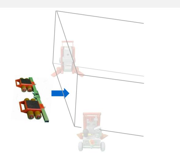
**Step 2:** Slide the rear skates underneath the load, then lower the load onto the skates.
