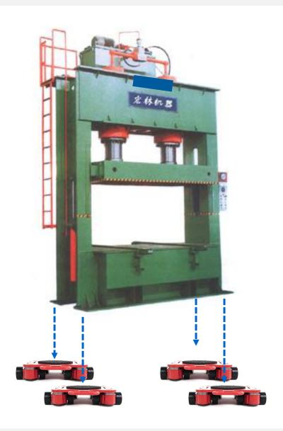
Heavy loads exert such high pressure onto the rollers that traditional rollers have a difficult time turning into a new direction. Often crow bars must be used to turn the rollers.
