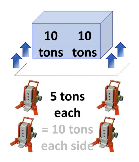
And if you are going to lift-up all 4 corners at the same time, each jack must carry 5 tons. So use four 5-ton jacks to carry the total weight of 20 tons.
