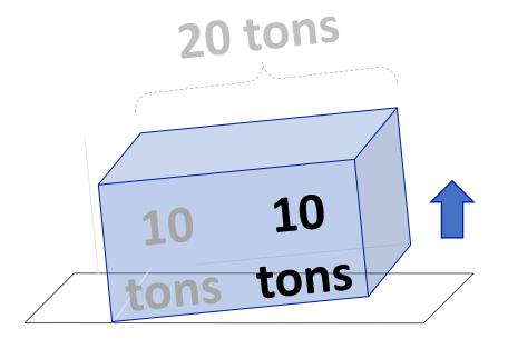
The weight to be lifted on each end is therefore 10 tons - or half the total load weight.
