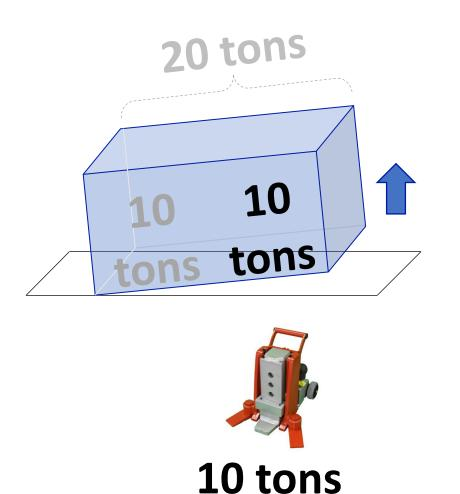
So, if you are planning on using one single jack, use a jack with 10 tons of lifting capacity.
