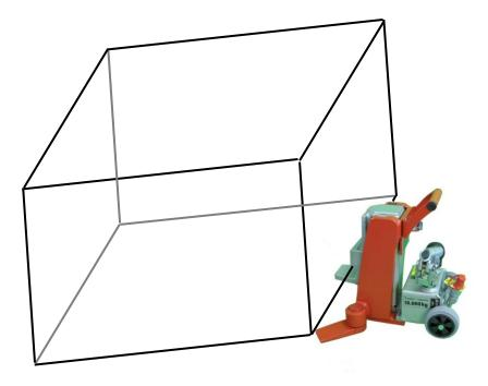
First, determine how many jacks you are going to use. The most economical solution is to use one jack to lift-up one end of the load at a time.
