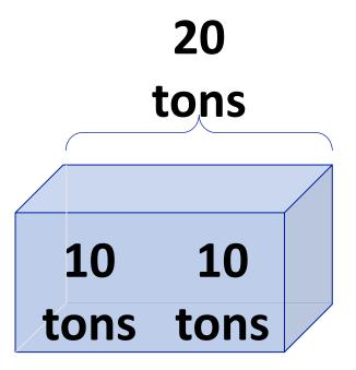
Then divide the weight equally into 10 tons on each end of the load.
