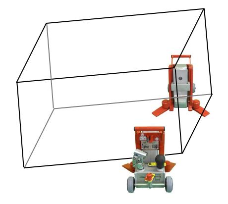
Or use 2 jacks simultaneously to lift-up one end of the load. This is often more convenient because it provides more usable clearance underneath the load.
